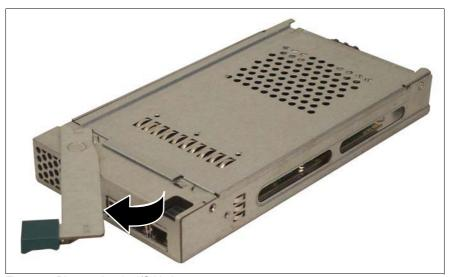
Figure 48: Disengaging the I/O blade
